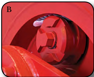
Rotary cable anchor for easy installation from either direction.
